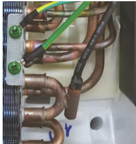
The Coil Temperature Sensor is a negative coefficient thermistor that will decrease in resistance with increases in coil temperature. The sensor is located in a socket soldered to the surface of the indoor coil.
