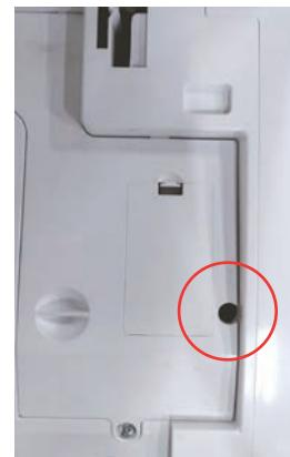
If the remote control is non-functional, the Emergency Button can be accessed by swinging open the front of the wall unit. The button is located on the right side.
