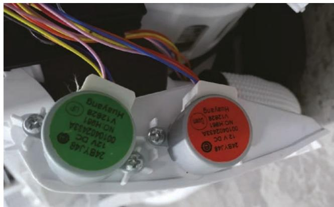
The STEPPER MOTOR moves the louver up or down, and right or left depending upon selections made at the remote control.
