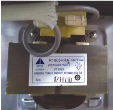
The Reactor is an inductive filter that will aid in correction of electrical power factor influence of inverter capacitance. It is unlikely to ever have an electrical failure of this component.
