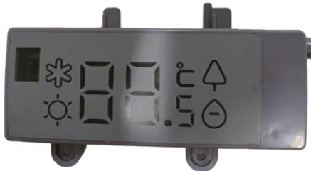
The indoor display has an infrared communication circuit that receives operating commands from the remote control. This display will indicate operating modes, error codes, indoor air temperature, timer status and power status.
